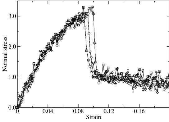
FIG. 3. Plots of the stress-strain behavior of different sized system I, which are being strained at a rate of  $\dot{\epsilon} = 3.1 \times 10^{-5} \tau^{-1}$ . Each curve represents a different sized system:  $N = 30\,000$  ( $\square$ ),  $60\,000$  ( $\diamond$ ),  $120\,000$  ( $\circ$ ) particles.
