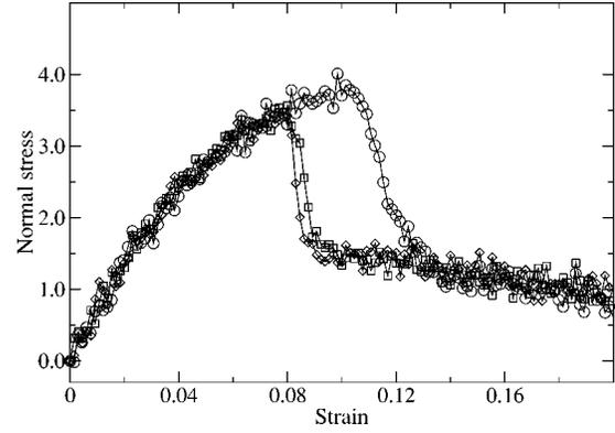
FIG. 5. Comparison of different strain rates on the strain behavior of system II. Each curve represents a different strain rate:  $\dot{\epsilon} = 3.1 \times 10^{-4} \tau^{-1}$  ( $\circ$ ),  $\dot{\epsilon} = 3.1 \times 10^{-5} \tau^{-1}$  ( $\square$ ), and  $\dot{\epsilon} = 3.1 \times 10^{-6} \tau^{-1}$  ( $\diamond$ ).
