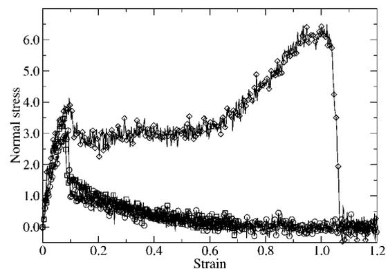
FIG. 1. Comparison of the stress-strain behavior of system I ( $\circ$ ) and system II ( $\square$ ) mixtures of monomers, when a strain rate of  $3.1 \times 10^{-5} \tau^{-1}$  is applied to each system. A typical stress-strain behavior of a highly cross-linked epoxy system (from Ref. [1]) is also shown ( $\diamond$ ).
