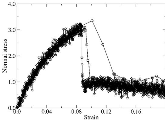
FIG. 4. Comparison of different strain rates on the strain behavior of system I. Each curve represents a different strain rate:  $\dot{\epsilon} = 3.1 \times 10^{-4} \tau^{-1}$  ( $\circ$ ),  $\dot{\epsilon} = 3.1 \times 10^{-5} \tau^{-1}$  ( $\square$ ), and  $\dot{\epsilon} = 3.1 \times 10^{-6} \tau^{-1}$  ( $\diamond$ ).
