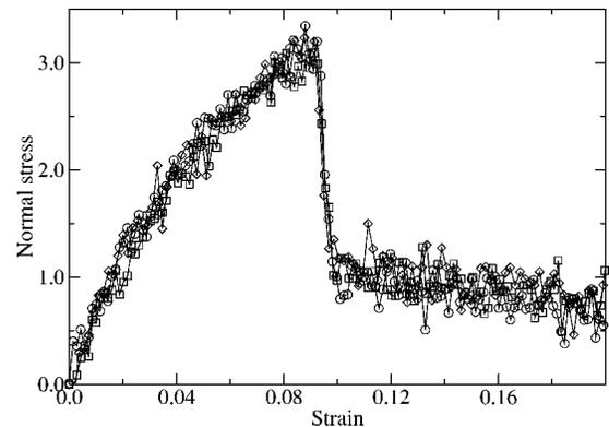
FIG. 6. Plots of the stress-strain behavior of system I samples that experienced a temperature drop of  $\Delta T_q = 2.0$  ( $\diamond$ ),  $3.0$  ( $\circ$ ), and  $4.5$  ( $\square$ ) during the quench and then were strained at a rate of  $\dot{\epsilon} = 3.1 \times 10^{-5} \tau^{-1}$ .
